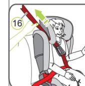
6. Guide the diagonal seat belt section 16 into the dark red belt holder 01 of the headrest 22 until it lies completely in the belt holder 01 and is not twisted.
