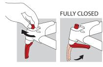
To properly close the quick release and secure the rear wheel in the dropouts, confirm the axle is fully inserted in the dropout, while maintaining the wheel in this position, rotate the quick release toward stroller and into the FULLY CLOSED position.
