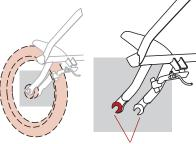
**Dropouts** (Secondary Retention Devices)
