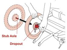
4. Adjust Quick Release Cam Lever To adjust the quick release, hold the quick release cam lever in the FULLY OPEN position with your right hand, and tighten the tension adjusting nut with your left hand until it is finger tight against the dropout.
